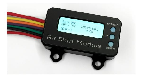
**Important** – leave the shift solenoid connector unplugged until you have configured the shift input polarity and verified correct operation!
