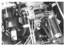
Start up the engine and keep it running at 1 300 rpm by turning throttle stop screw ③.
