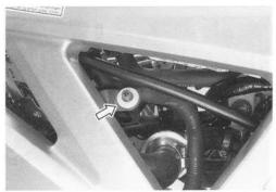
· Loosen the throttle body clamp screws.
