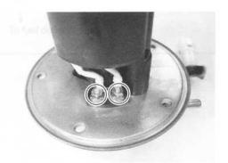
· Remove the screws and fuel level switch.
