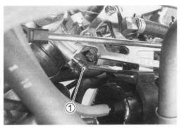
Connect the vacuum balancer gauge hoses to the vacuum nipples ② respectively.
