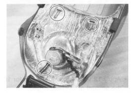
· Remove the fuel pump assembly by removing its mounting bolts diagonally.
