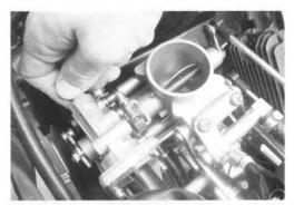
. If the TP sensor output voltage is out of specification, turn the fast idle adjusting screw 1 and adjust the output voltage to specification.
