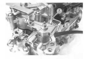
• Apply SUZUKI SUPER GREASE to the seal lips.
