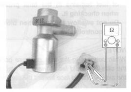
If the resistance is not within the standard range, replace the PAIR control solenoid valve with a new one.
