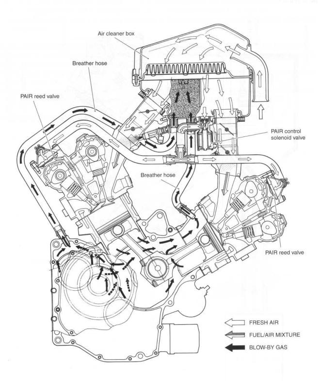
The exhaust emission control system is composed of the PAIR system.
