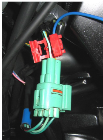
Figure 1 - 9 : Gear Position Sensor wire tap on Kawasaki ZX14
