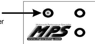
We generally start at around 75 ms. of kill time. The Kill Time is adjusted via a small potentiometer accessed through the grommet on the front of the unit. Using a small screwdriver Carefully turn the pot
