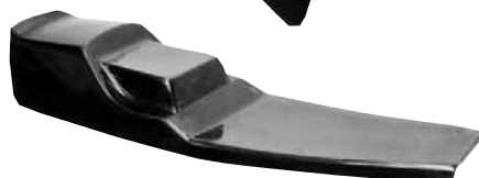
#49 SEAT TAILSECTION - TIRE AREA 6.5" WIDE OVERALL LENGTH 33.5"
