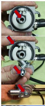
18. Refer to tables on page 1, install the proper high-altitude jet in the carburetor,
