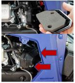
25. Place foam element back in the air box and replace the lid with the two bolts.
