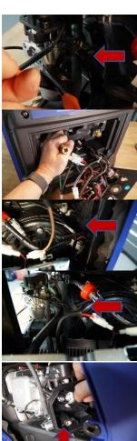
21. Reinstall the gasoline fuel hose on to the carburetor.
