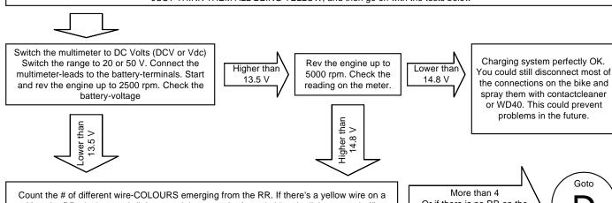
Count the # of different wire-COLOURS emerging from the RR. If there's a yellow wire on a Yamaha RR, don't count it (it is a special output-wire for switching the lights on and off)
