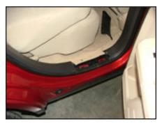
**STEP 5**Remove passenger side threshold plate.
