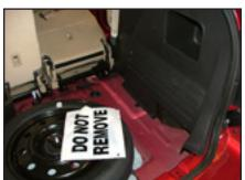
Remove foam filler panel or plastic storage tray from passenger side of spare tire.
