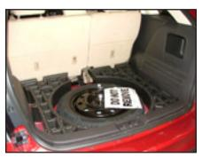
Remove the floor panel by lifting seat flaps. Carefully tilt entire panel to exit hatch diagonally.
