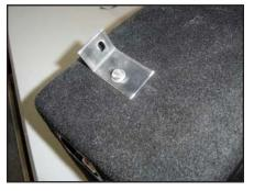
**S T E P 1 3**Attach the L Bracket to the top of the Stealthbox® using a 1/4"-20 x 1 Bolt, a 1/4" Lock Washer, and a 1/4" Flat Washer, as shown, and hand tighten.
