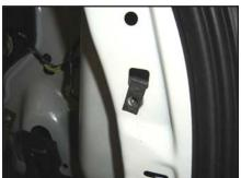
STEP 8 Insert a 1/4"-20 U-Nut into the square hole near the weatherstripping as shown.
