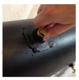
Thread in your 1/2"x1/4" fitting into one of the ports on the front of your air tank. This fitting will supply air to your paddle valves.
