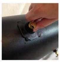
Thread in your 1/2"x1/4" fitting into On the neighboring port, plug it off one of the ports on the front of your using the supplied fitting and air tank. This fitting will supply air to tighten with a Hex Key. You will your paddle valves. tighten with a Hex Key. You will not need to use this port.
