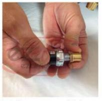
First, thread the pressure switch to the 1/4" reducer bushing. (don't forget the EZ Tite)
