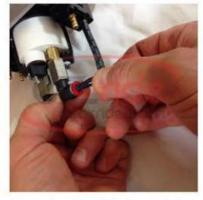
Next, plug the 1" air line strip from the Tee to the Red Head gauge fitting.
