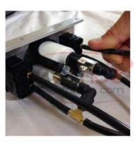
Now, plug 2 more strips of air line into the delivery barbs on the back of the gauge labeled "SUP." These barbs will "supply" air to your bags.
