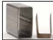
Cut-away view of Morrison's 2"x4" frame vs. OEM stamped rail
