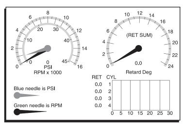
Figure 14 RPM and Retard Monitor.
