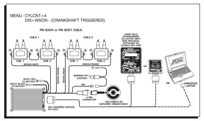
Figure 10 4-Cylinder Dual Spark Plug System Wiring WSON (Waste Spark).
