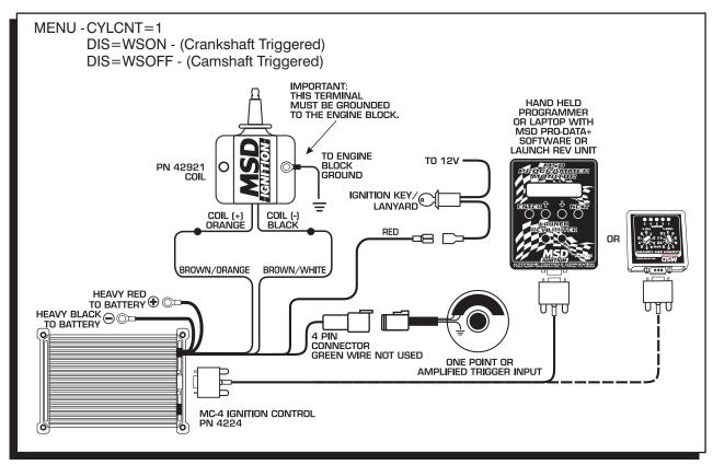
Figure 11 Single Cylinder Wiring.
