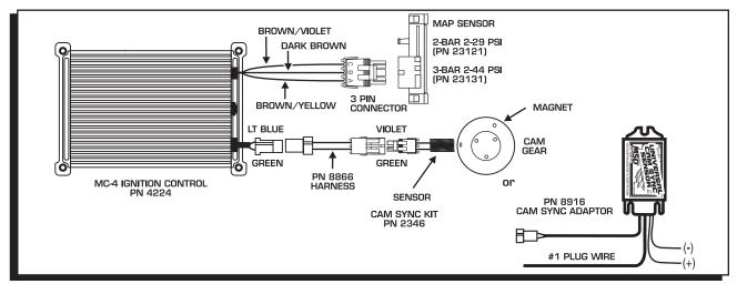
Figure 13 Using a Sync Signal or Map Sensor.
