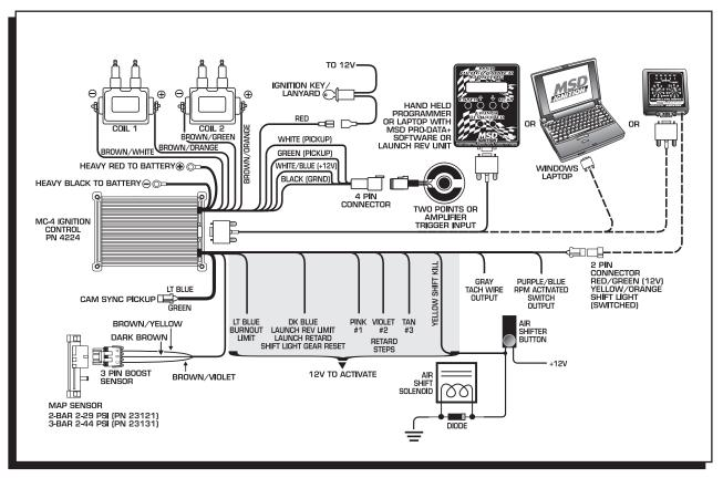
Figure 9 4 - Cylinder Single Plug WSON (Waste Spark ON - Crankshaft Triggered). 2 - Cylinder Dual Plug WSOFF (Waste Spark OFF - Camshaft Triggered).
