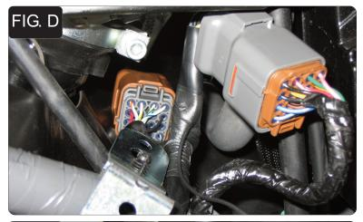
5 Connect the PCV in-line of the stock wiring harness and throttle body harness (Fig. D).
