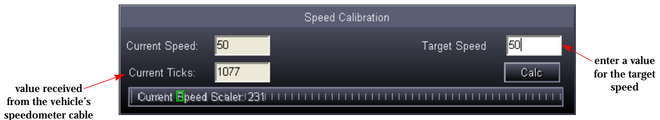
Figure 3-17: The Speed Calibration Dialog Box
