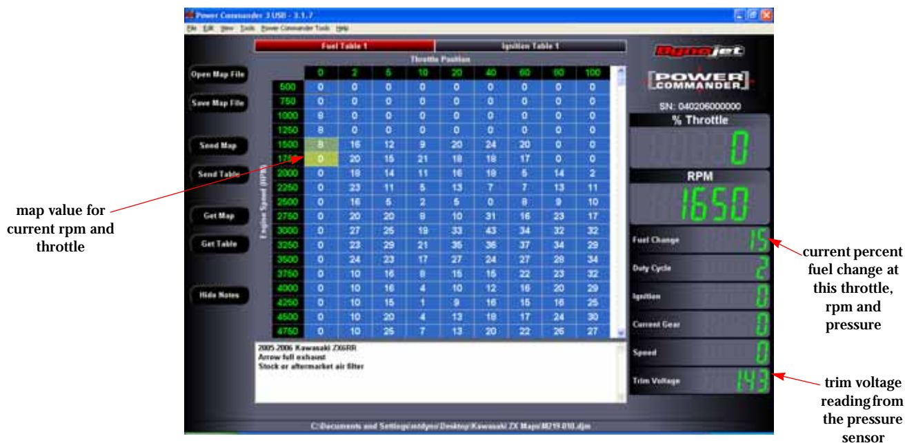
Figure 3-23: Pressure Trim Values Are Added to Fuel Adjustment Already in Map
