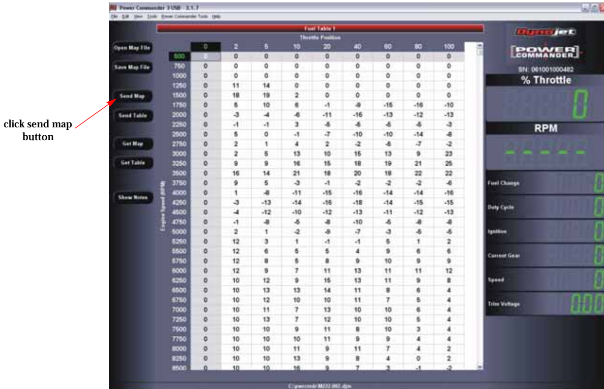
Figure 2-24: Use the Send Map Button to Transfer the Open Map to the PCIII USB
