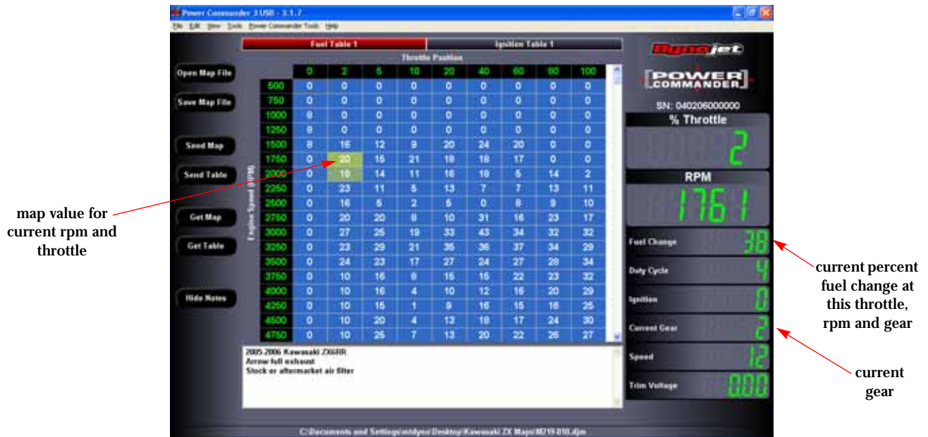
Figure 3-21: Gear Trim Values Are Added to Fuel Adjustment Already in Map
