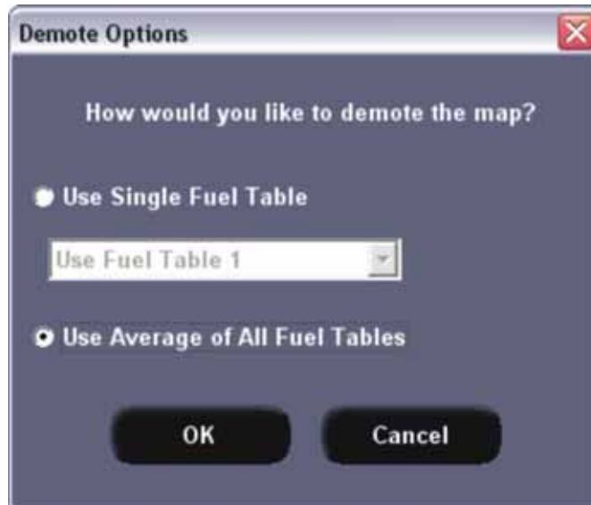
Figure 3-3: Demote Map to Basic Using the Averages of the Values
