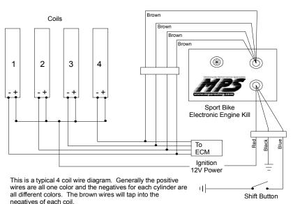
Horn Control Harness) **Control Box Wiring** Coils - Most four cylinder motorcycles use either a individual firing system or a waste spark system. Waste spark is by far the most common. All four cylinder bikes with only two coils use a waste spark system. Most late model four cylinder sport bikes use waste spark systems even though they have four individual coils. Some of the newest fuel
